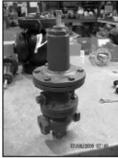
Remove valve from line.
