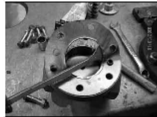
Remove any residual gasket material.
