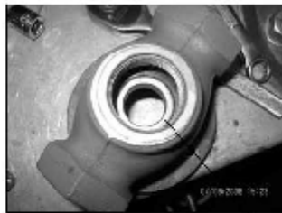
Inspect sealing surface on seat in valve body.
