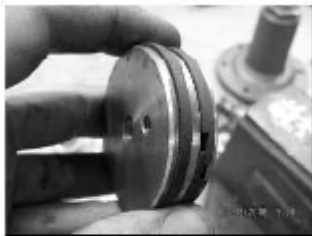
Push piston out of body and inspect rings and body bore.
