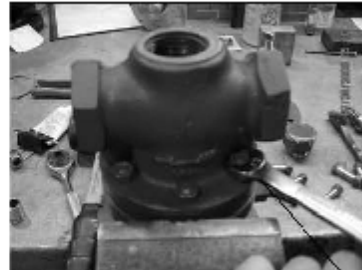
Invert assembly in vise to remove pilot body bolts.
