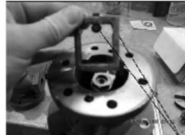
Remove pilot yoke & disc from pilot body.
