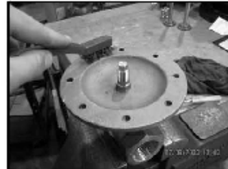
Clean sealing surfaces.
