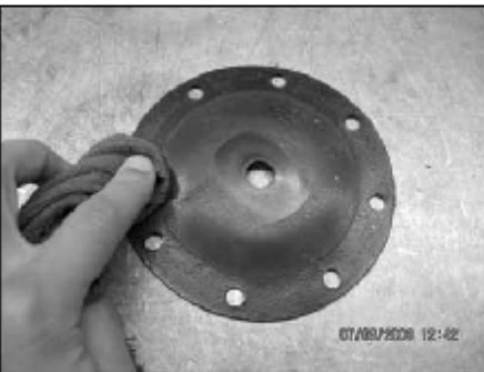
Clean & inspect diaphragm.
