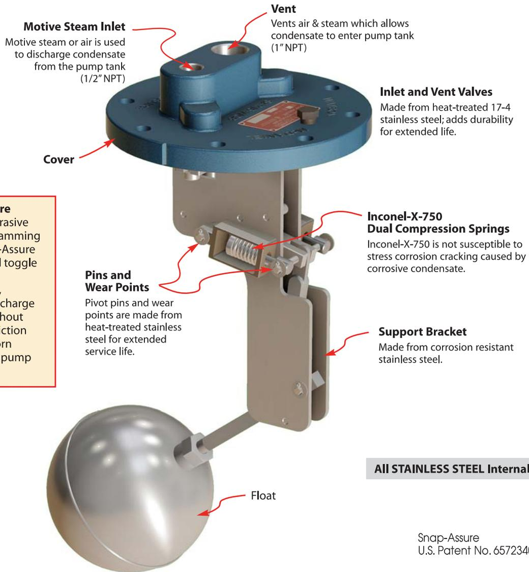
**The Patented Snap-Assure Feature** stops dirt and abrasive iron oxide particles from jamming the mechanism. The Snap-Assure Feature forces the internal toggle action to trigger ("snap") between vent and motive, "assuring" that fill and discharge cycles occur properly. Without Snap-Assure, the added friction of abrasive particles or worn components can inhibit a pump from operating.
