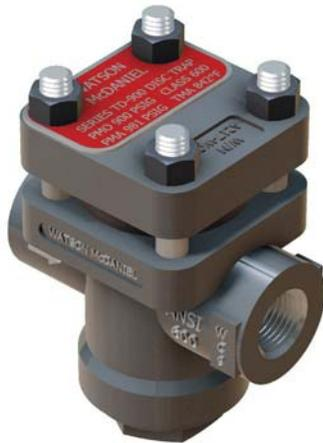
The **Thermodynamic Disc Trap** is simple and compact and an excellent choice for a wide variety of drip applications. They excel in drip applications of pressures ranging from 30 psig to high pressure applications exceeding 3,000 psig, including superheated steam. The ½" TD600L is suitable for most drip applications, and offers reduced size discharge orifice holes which are preferable in terms of performance, longevity, and efficiency.
