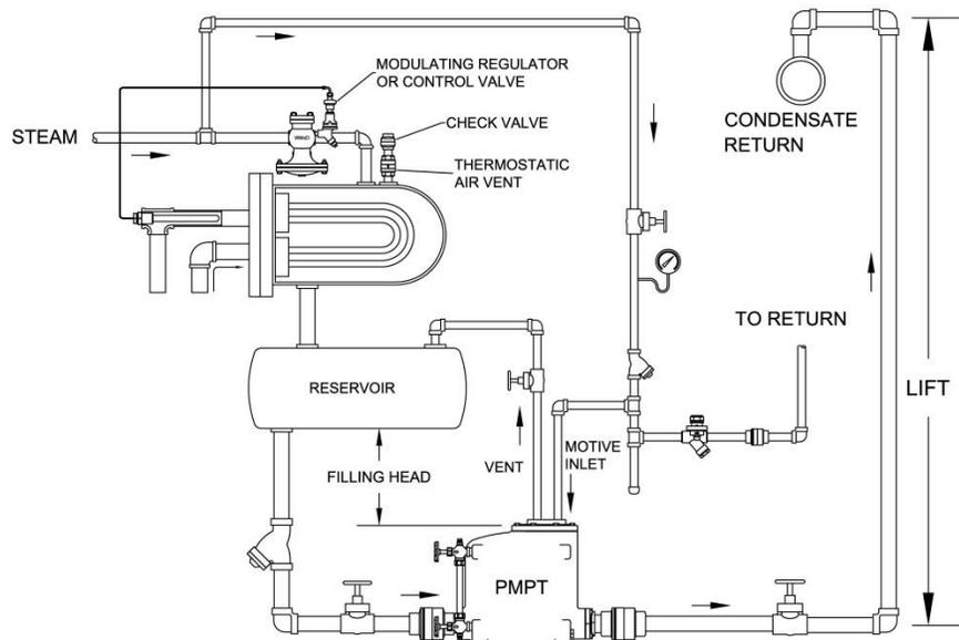
Figure 4: Closed Loop Pump System
