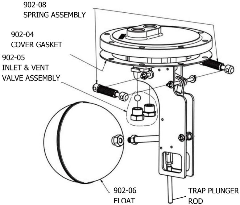
**Figure 7: 912-03 Complete Pump Mechanism for PMPT**
