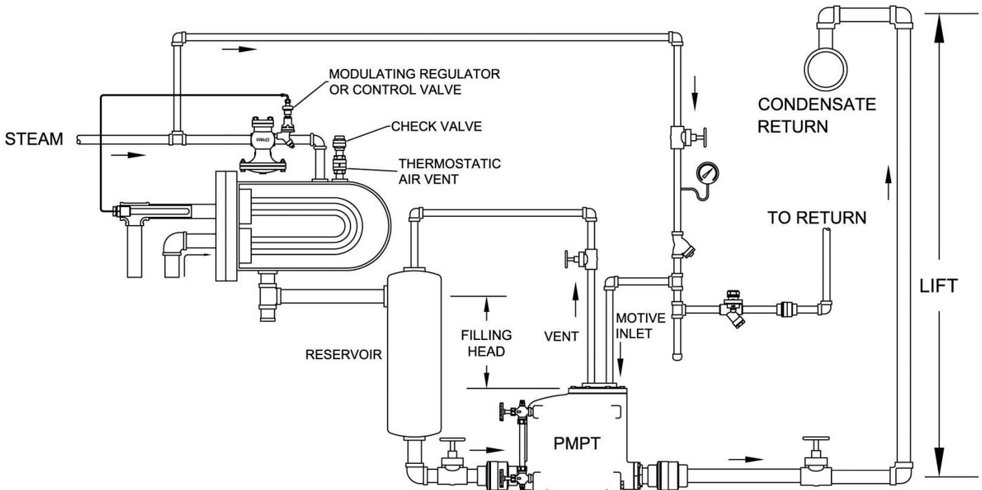
**Figure 5: Closed Loop Pump System with Vertical Reservoir when Fill Head is Restricted**
