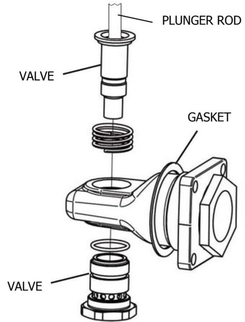
**Figure 8: 917-03 Internal Trap Assembly Mechanism for PMPT**
